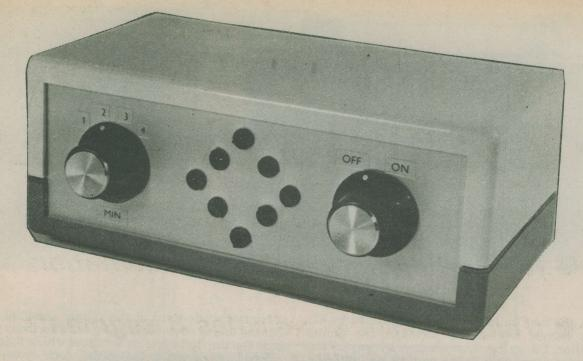
The ring of l.e.d.'s appears on the front panel of the timer. The top l.e.d. lights up at the start of the timing period, then extinguishes as the next l.e.d. turns on. The l.e.d.'s become illuminated in turn in clockwise order and the timing period is at an end when the eighth l.e.d. gives way to the first one in the ring
